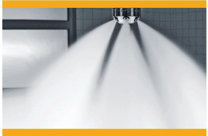
**Marioff HI-FOG® systems fight fires just as effectively as traditional sprinkler systems, but with significantly less water. Dispersing water as small droplets, a HI-FOG® system cools a fire and its surroundings, blocks the fire's radiant heat and eliminates oxygen from the seat of the fire.**
