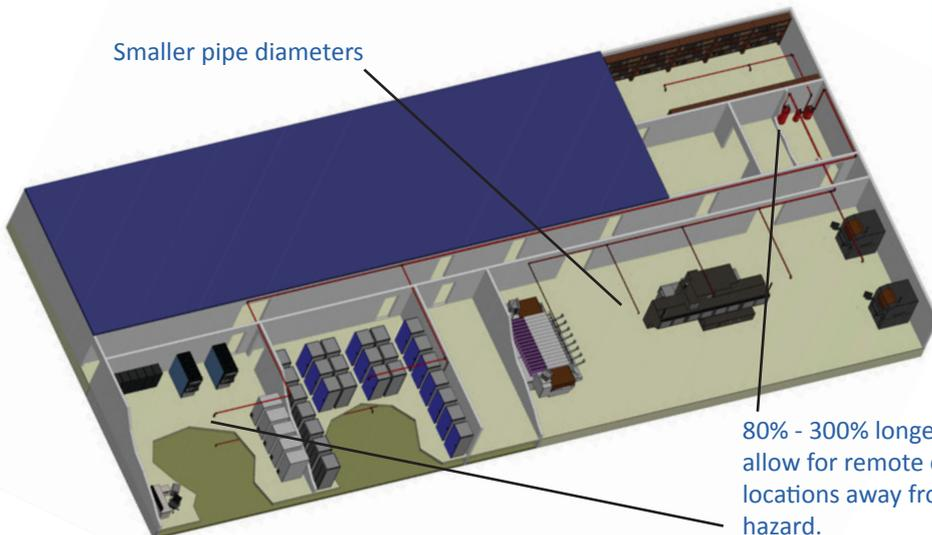
80% - 300% longer pipe runs allow for remote cylinder locations away from protected hazard.
