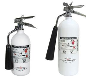
**CARBON DIOXIDE** is discharged as a white cloud of “snow” which smothers a fire by eliminating oxygen. It is effective for Class B flammable liquids and is electrically non-conductive. Carbon Dioxide is a clean, non-contaminating, odorless gas.
