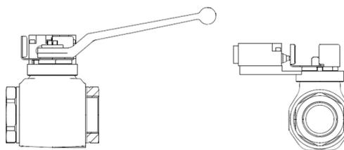
Figure 14. Lockout Valve
