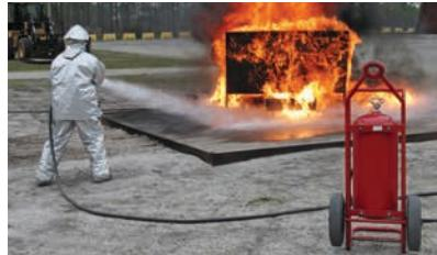
The new Amerex Model 775 is UL-listed with a 3A:80B:C rating. Shown here is a test unit used to obtain UL approval. The actual unit is similar to conventional Halon 1211 units, making the transition to the Novec 1230 fluid based Model 775 easier.
